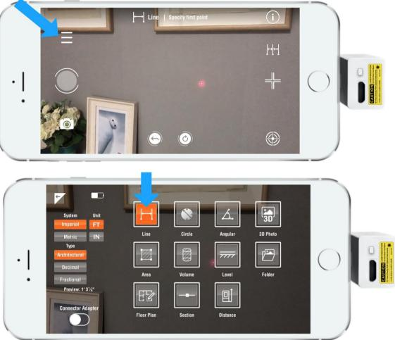
Aim the laser dot to the start of the line, and tap Measure button. A virtual dot will be placed there.
