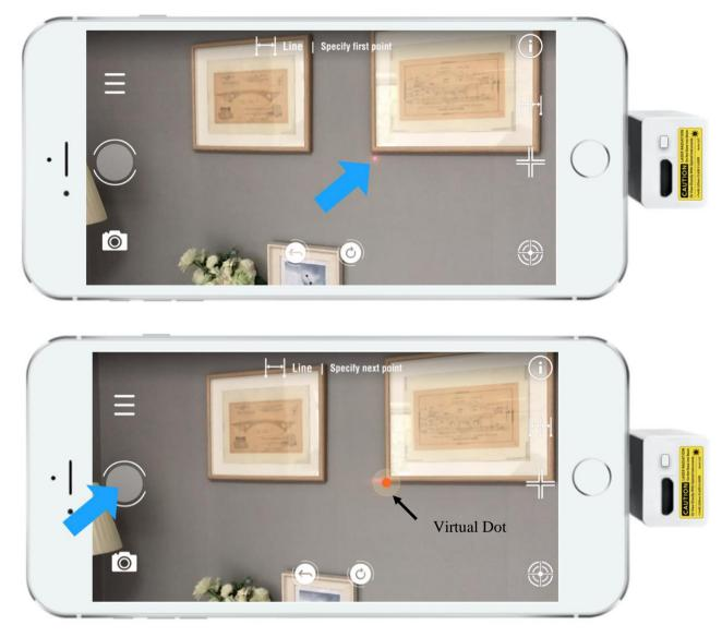
Aim the laser dot to the end of the line, and tap Measure button again, another virtual dot will be placed, and the measurement result will be shown.
