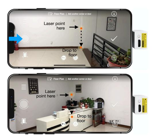
laser beam, and tap **Measure**, the point will automatically drop down to the floor.
