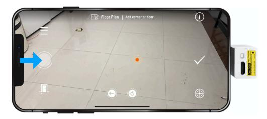
Point the laser to first corner and tap **Measure** button. If there is obstacle, you can move up the
